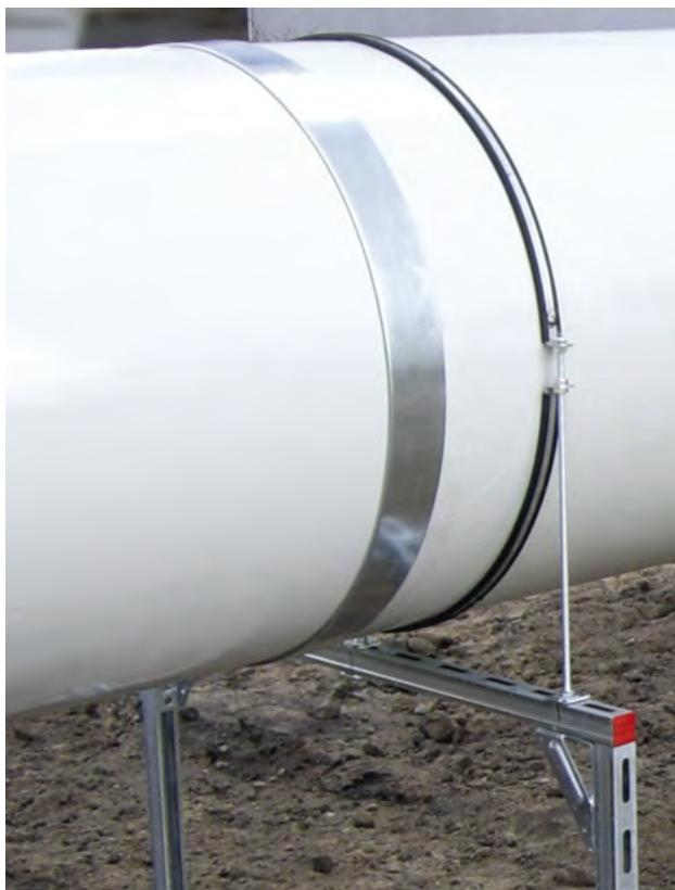
**Proven two-part construction for fixation at the closing flap.** Designed for the dimensions of the VENTAFLEX® air duct system. Safe fixing by means of thread rods due to the M10 through holes of the closing flaps. Fullfills the requirements of thermal decoupling.
