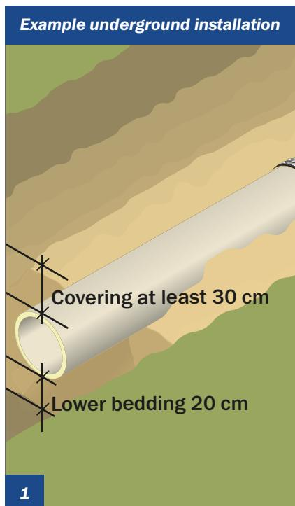
Before installation a ditch must be made which guarantees a 20 cm support and a covering of at least 30 cm of filling sand.
