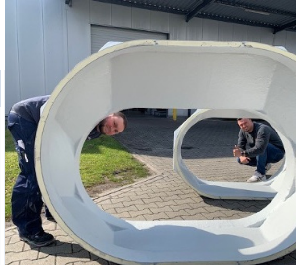
Our technicians proudly present their "giant babies": custom-made special components, in this case reductions of various diameters
