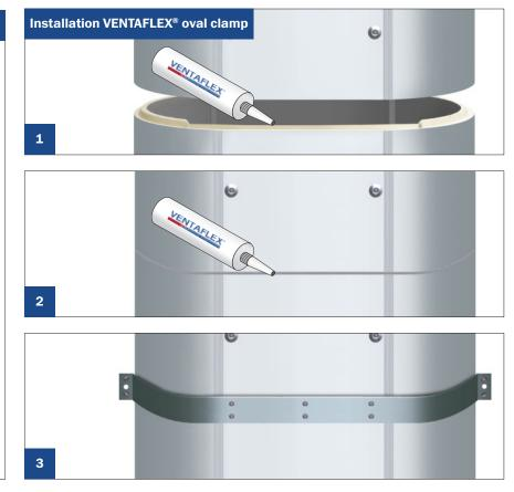
Apply the glue on the different planes of the connection points. Attention has to be paid that all adhesive- and seal surfaces must be freed from dust, grease and other deposits.
