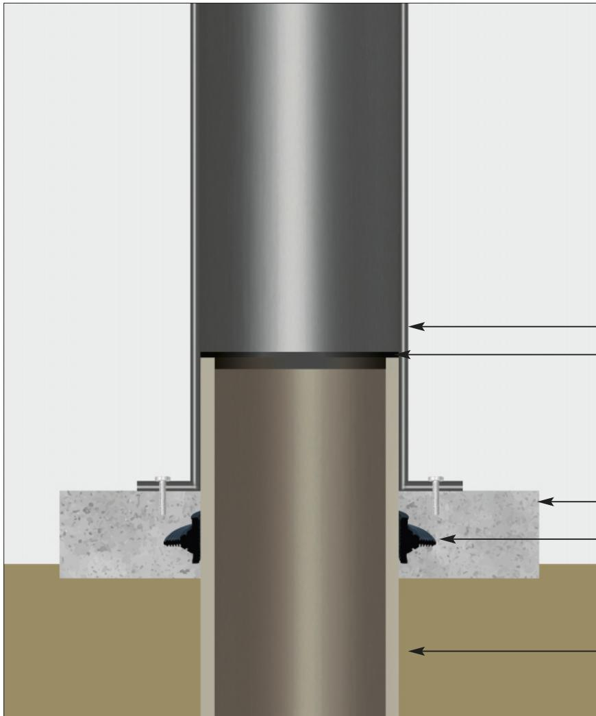
There are many different possibilities to connect an air duct to ventilation towers. This exemplary illustration shows the installation of the LAVANTUS® air duct to a ventilation tower by inserting it through a wall collar in the base plinth. (see installation instruction wall collar). In the example the ventilation tower is put on the protruding end of the air duct and attached to the base plinth.
