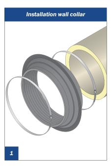
Push the wall collar onto the LAVANTUS® air duct with both clamping rings.
