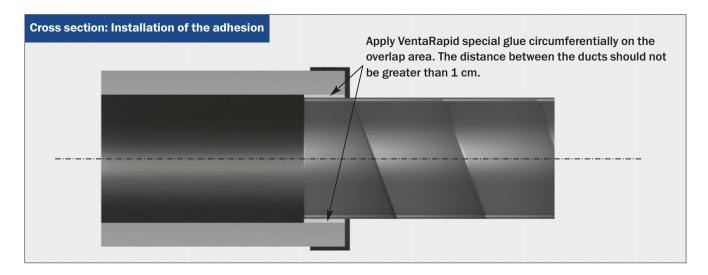
Since the diameters of the ducts of other producers are very often similar to the ducts of the VENTAFLEX® system, absolutely tight connections can be produced uncomplicated. A fitted cut-out end cover – if requested – makes an optically clean completion.
